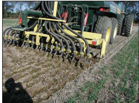
Figure 1 Aeration tillage loosened the soil, conserved crop residue, increased surface roughness and improved infiltration of the manure. Spring no-till planting was not a problem.
